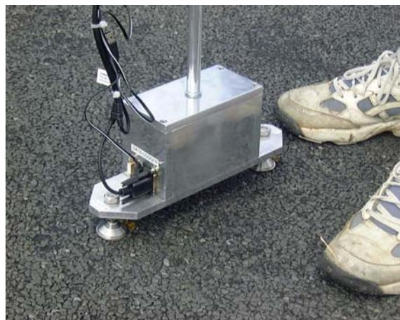
**Figure 1: ROMDAS z-250 Stationary Inclinometer.**
